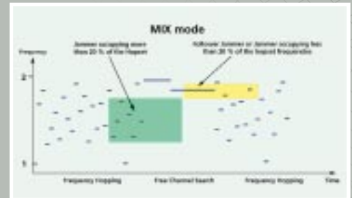
Fig. 1: In mixed FH&FCS mode, radio automatically selects the more appropriate mode, FFH or FCS, according to EW environment.
